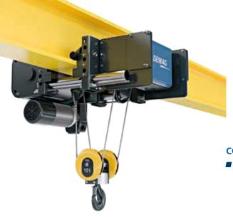
The special trolley configuration is suitable for a variety of girders. It minimizes the overall height of the crane from the top of the crane structure to the lifting hook. This helps to reduce the vertical space needed for crane movement and safety clearances in the building.
